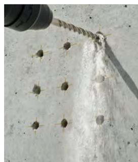
This level of efficiency is achieved through the combination of an innovative drilling head and large-sized flutes which prevent stoppage of the drill bit.
