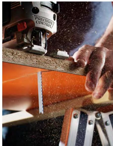
The **cut quality** is directly related to the **geometry** of the saw blade.
